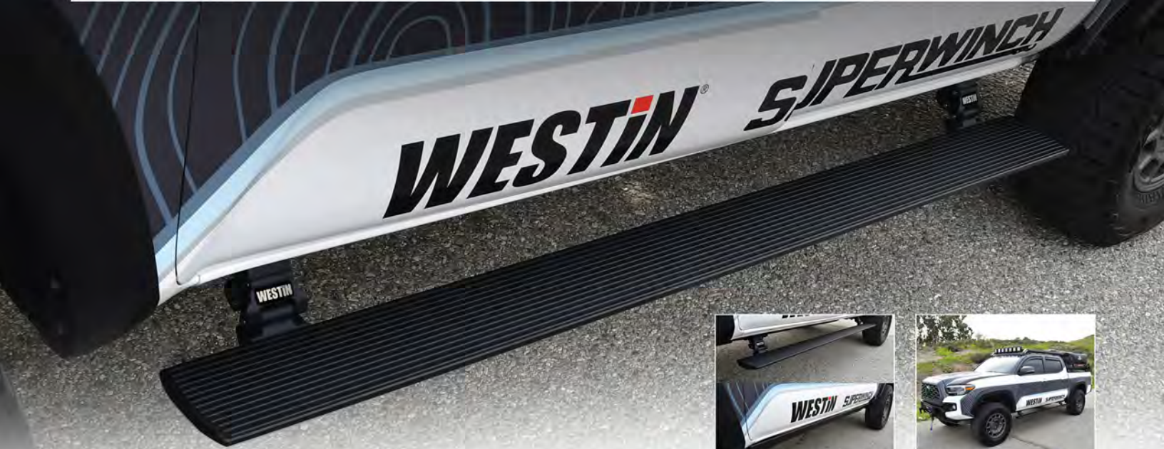
Pro-e Power Running Boards shown open and closed
