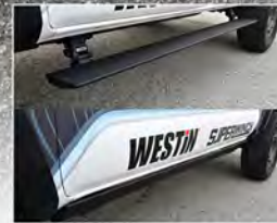
Pro-e Power Running Boards shown open and closed
