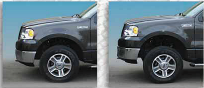
BILSTEIN 5100 Series Leveling Shocks offer multiple spring seat positions for ride height adjustment ranging from stock height up to 2.75", depending on the application.
