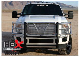
Westin's New HDX Grille Guard is made of a 1-piece welded construction with interior and support light guard brackets made of 1" tube. Uprights are fully lined with 1/8" thick and 2" wide rubber to protect the grille guard from bumps and scrapes at the outer most part of the uprights. The HDX Grille Guard also features a full punch plate center grille to intercept impact from flying debris.
