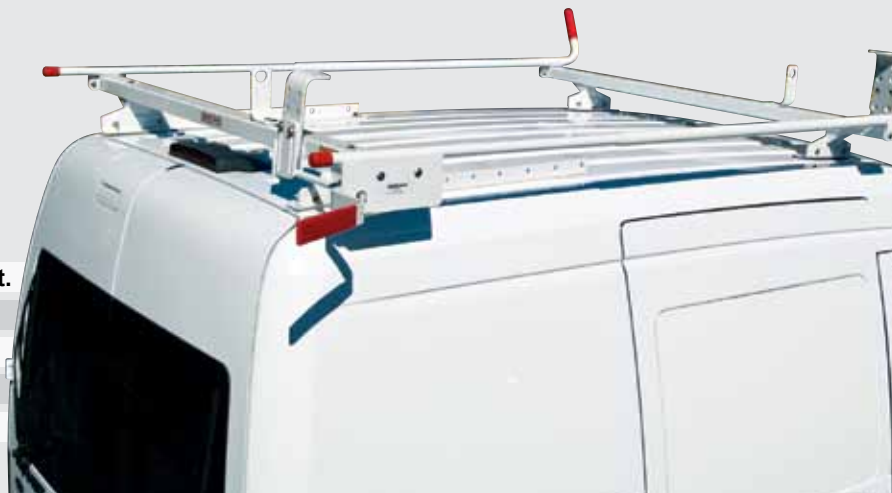
Adjustable roof rack accommodates variable sizes of ladders and materials
