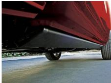
**DOOR CLOSED** - Retracts safely under the vehicle with no loss of ground clearance.
